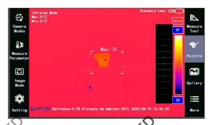
SATINFRARED Adjust the lower setting -Span (Note bottom highlighted in blue) If the top temperature is highlight, then it will adjust the top value.
